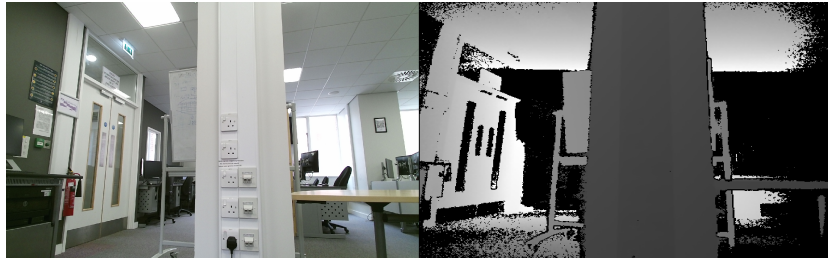
Figure 19: Depth images from the Xbox sensor, left normal image, right depth image.
