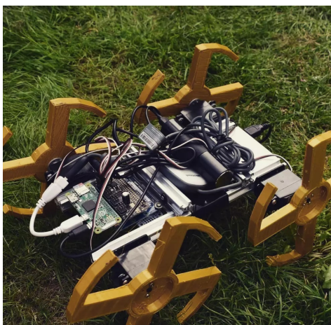
Figure 1: Prototype of the Whieg robot to test out the whieg design, in addition the hardware required. This prototype ran on a Raspberry Pi zero and used a phone charger cell providing 5.1V and a maximum of 2A of current.
