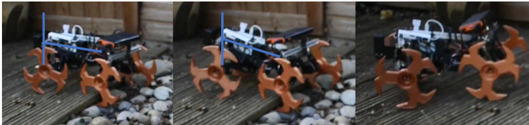
Figure 40: How the angle on the robot changes with back actuation. The first image is where the robot got stuck going over a barrier. The second image shows the distribution of weight to the centre of the robot, which allowed more torque to be focused on the back wheel rotation rather than holding the weight of the robot. The final image shows the robot having climbed over the obstacle. Outlined in Figure 40 is a drawn axis in blue to demonstrate the movement undertaken by the robot.
